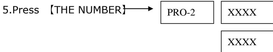
The number is related to step 4. For example, to calibrate 30 kg scale with a 10 kg standard weight, press 【3】 ; to calibrate with a 30 kg standard weight, press 【1】 .
